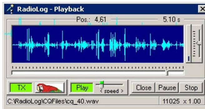
With this option and some additional hardware, CQ calls can be automatically repeated. The hardware consists of an interface (for connecting the sound card, the serial port, and the microphone) and a connector cable to the microphone and headphone jacks of the transceiver.
